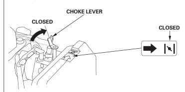
To restart a warm engine, leave the choke lever in the OPEN position.
