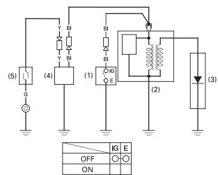
(1) ENGINE SWITCH(2) IGNITION COIL
