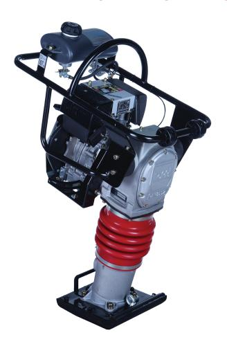
Rammer is light weight compaction equipment used for compacting small areas by providing impact load to the soil. This compaction equipment is light and can be hand operated or machine operated. Rammers are most suitable for ohesive and semi-cohesive soils. Due to light weight, it is used for interior floor compaction. It is also used for repair of road, shoulders, pavements, highways and street.
